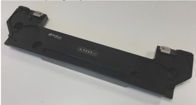
Figure 5: NORIA fiber fixture with integrated accurate pre-strain feature
