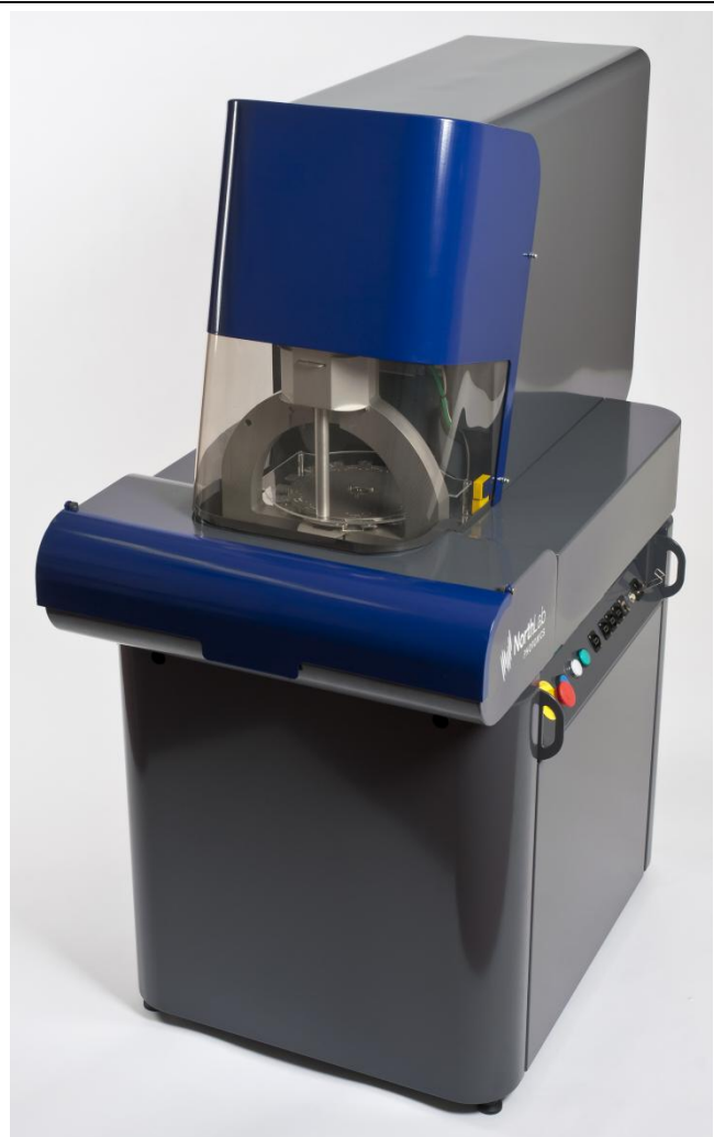
Figure 1: NORIA fiber Bragg manufacturing system
